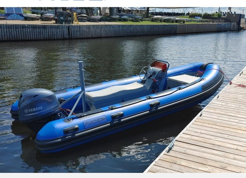
The PACE Pursuit range of commercial quality RIBS are purpose built to be tough workboats or high performance chase craft capable of withstanding the harshest conditions. Pursuit RIBS feature deep V, 4-5 mm aluminum hulls and large diameter tubes from quality European fabrics, making them ideally suited for use as support, safety, and coach boats. Our boats can be configured with a wide range of seating and console options, allowing you to design the perfect PACE RIB for your needs.
