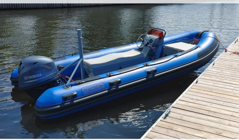
The PACE Pursuit range of commercial quality RIBS are designed to be tough workboats or high performance chase craft capable of withstanding the harshest conditions. Pursuit RIBS feature deep V, 4–5 mm aluminum hulls and large diameter tubes, making them ideally suited for use as support, safety, and coach boats. Our boats can be configured with a wide range of seating and console options, allowing you to design the perfect PACE RIB for your needs.
